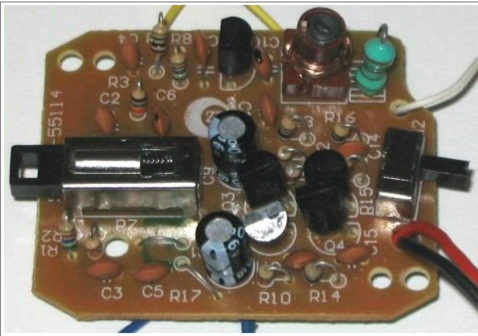
The 1/10th watt resistors used in this circuit, compared with 0.25watt resistors.
