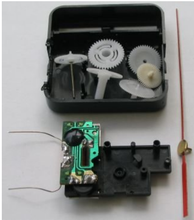
The crystal removed and a "cut track" to the coil. The 6 gears must be re-fitted for the hands to work.
