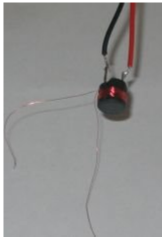
The 10mH choke with 150 turns for the secondary
