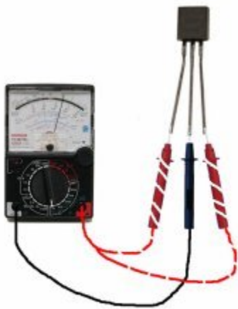
This is an NPN transistor The black probe is the BASE
