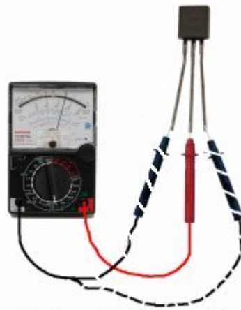
This is a PNP transistor The red probe is the BASE
